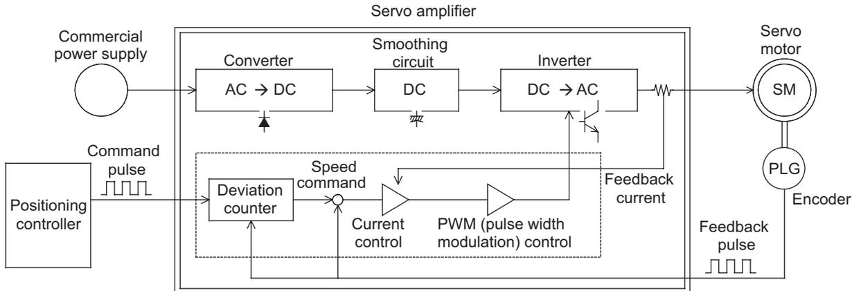
The positioning controller generates a specified quantity of forward rotation (or reverse rotation) pulses at a specified frequency.
